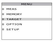
2. Press either or key to select [TARGET] and then press ENTER key.
